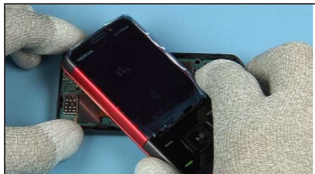
44. Gently lift up and flip the upper part over the D-COVER.
