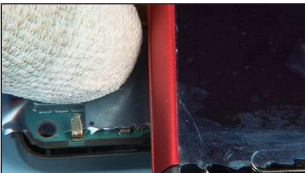
43. Use the tape to align the connector correctly. Close the connector and remove the tape.
