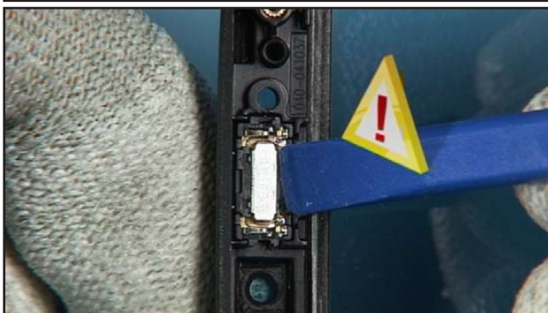
15. Push it down carefully. Never push down the metal part, otherwise the EARPIECE could be destroyed.
