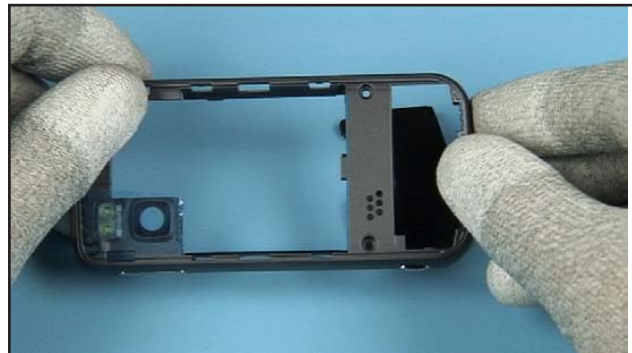
50. Turn the D-COVER. Simply let drop out the ANTENNA IHF ASSEMBLY.
