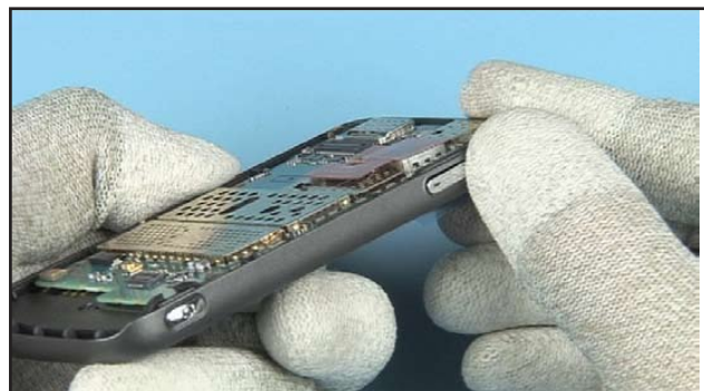
12. Check that all keys operate before going on.
