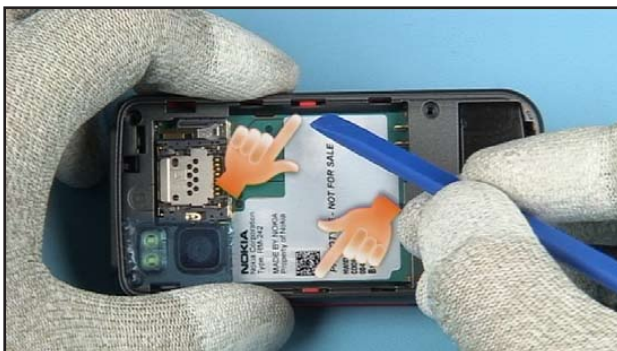
11. Unlock both clips of the A-COVER with the SS-93.
