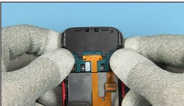
29. Carefully bend the A-COVER on both sides...
