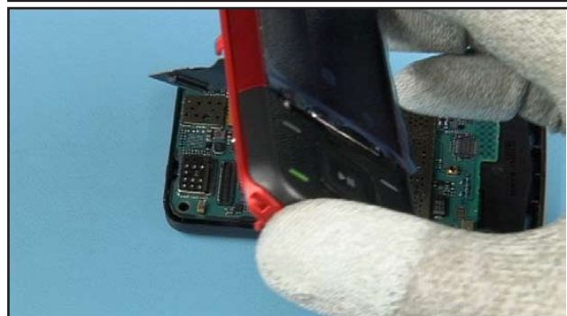
16. The assemblies can be separated now.
