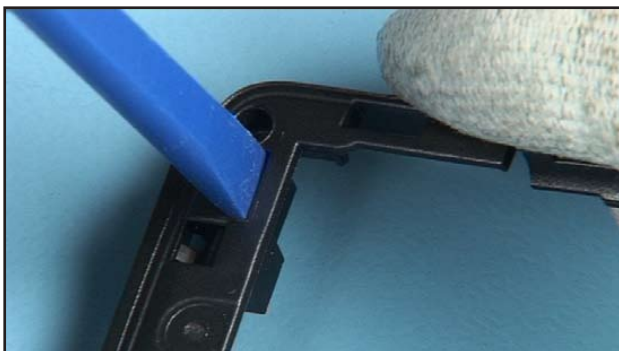
51. Push out the DC jack partly.
