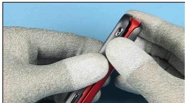
12. Slightly release the assemblies, beginning at the bottom side.
