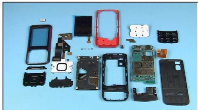
54. The disassembly procedure is now finished.
