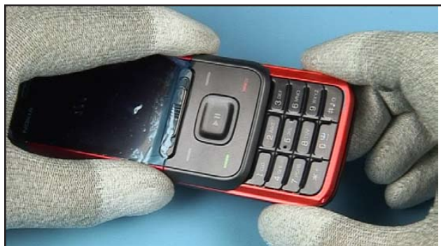
60. Check the correct placement of the keymat.
