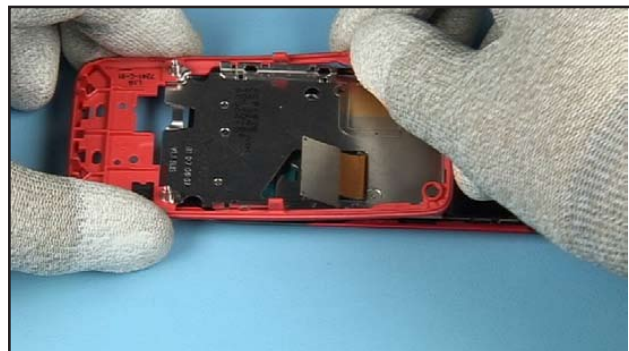
22. Carefully release the LOWER BEZEL ASSEMBLY from the metal snaps of the SLIDE MODULE ASSEMBLY.
