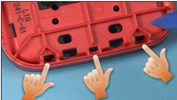
17. Unlock these 3 plastic clips with the SS-93.
