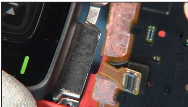
21. Keep this adhesive clean if this part should be used again.
