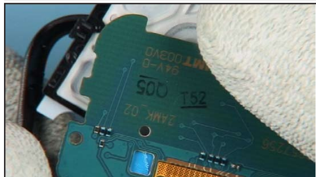
32. Lift up the TOP PWB. The TOP KEYMAT ASSEMBLY can be removed now.
