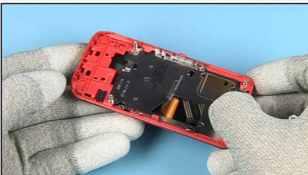
39. Check the functionality of the slider before continuing.
