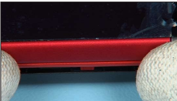
45. Click these clip into its place, -also at the opposite side.
