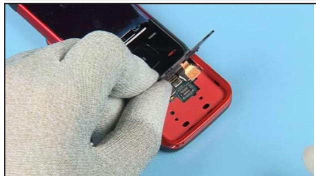
48. Bring the BOTTOM KEYMAT SUPPORT into position as shown.
