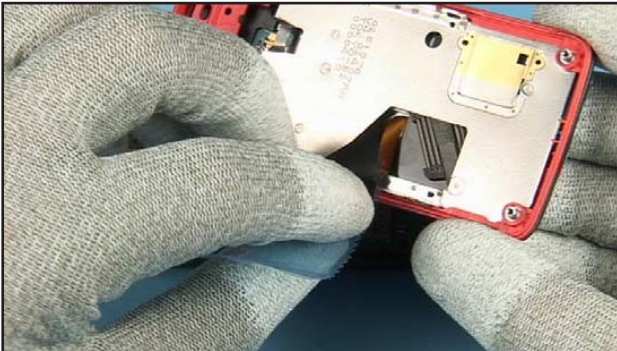
41. Carefully flip the flex foil as shown. Do not fold it!
