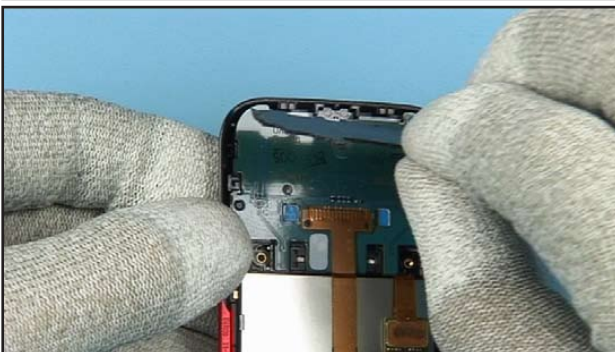
31. Lift up the NAVI KEYMAT SUPPORT.
