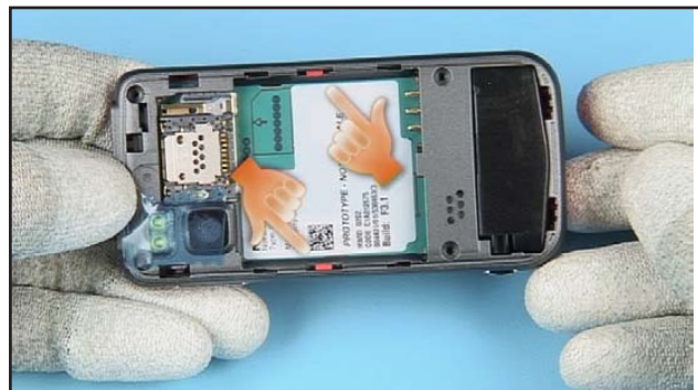
46. Check the correct positioning of both clips before going on.
