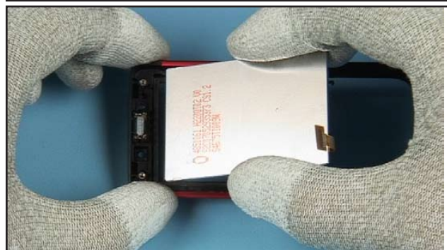
16. Align the LCD to the top guide. Smooth it down evenly.
