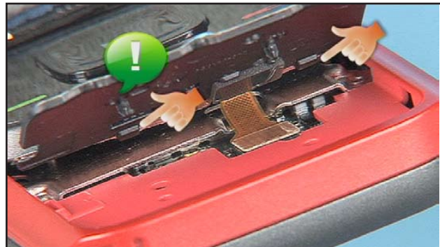
50. Align the shown plastic clips of the BOTTOM KEYMAT SUPPORT...
