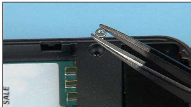
54. Close the slider. Insert the 4 new screws.
