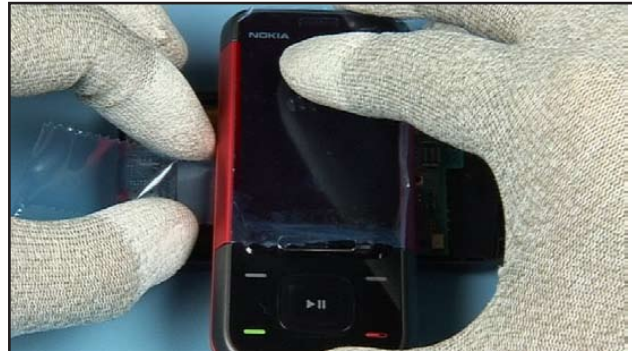
42. Hold the flex connector. Bring the upper part into position over the lower part as shown.
