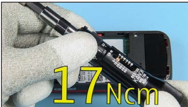
55. Set the correct torque.
