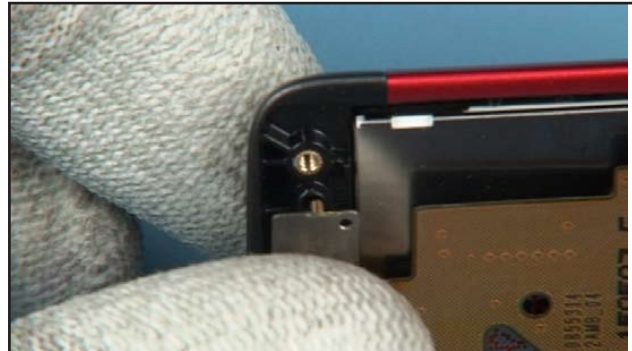
18. Slightly push the CMOS CAMERA and this guide pin into its place.
