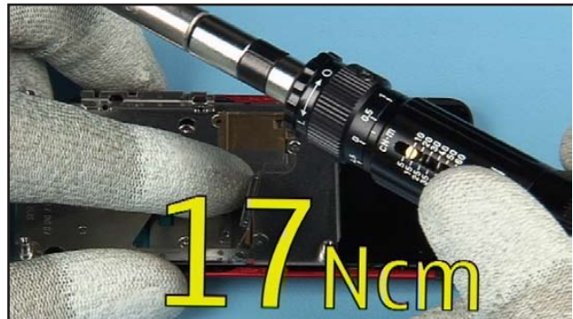
34. Set the correct torque.
