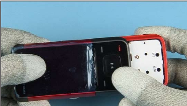
57. Shift open the assembly again.
