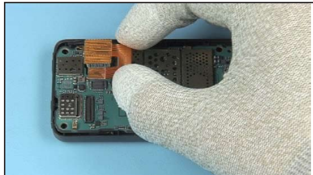
10. Check the camera window for cleanliness. Insert the CAMERA FLEX MODULE into its compartment.
