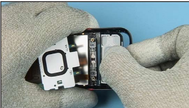
25. Fit the TOP KEYMAT ASSEMBLY into the A-COVER.
