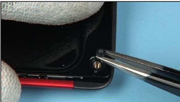
33. Insert the 4 new screws.
