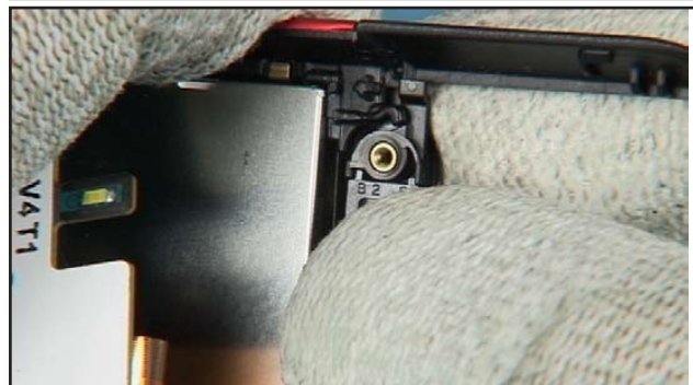
24. Click the clip on the opposite side into its place.
