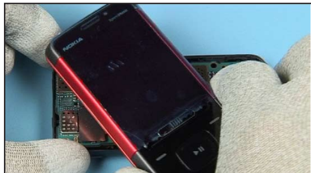
14. Gently twist the upper assembly near to 90 degree.
